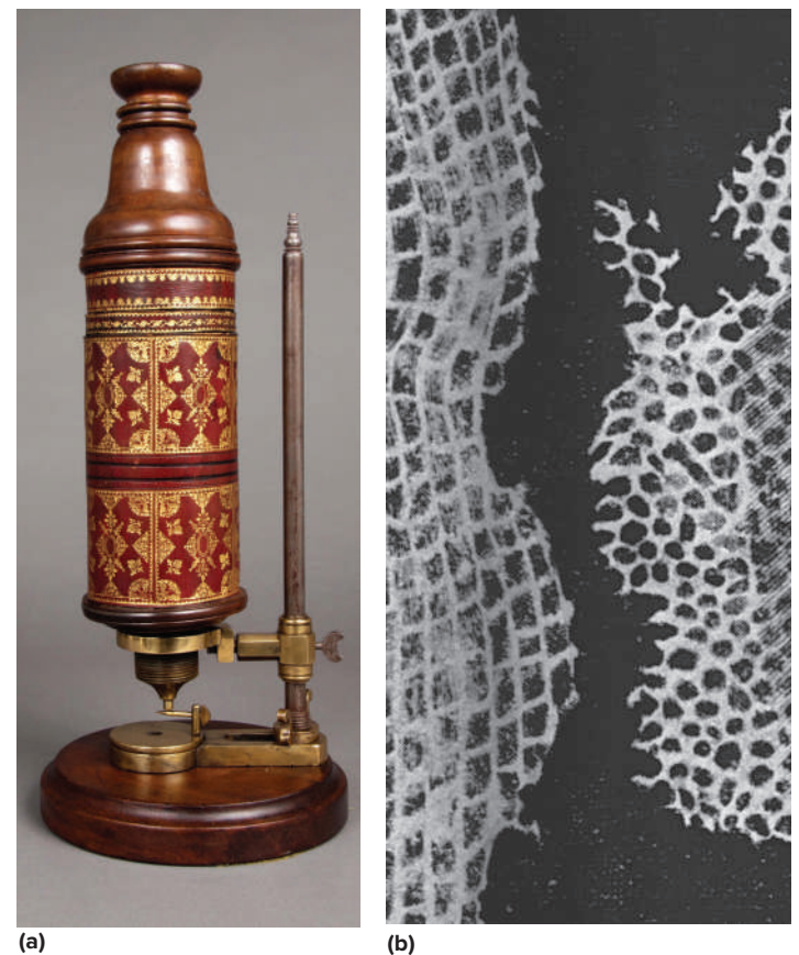
FIGURE 1.2 Hooke’s Compound Microscope. (a) The compound microscope had a lens at each end of a tubular body. (b) Hooke’s drawing of cork cells, showing the thick cell walls characteristic of plants.
